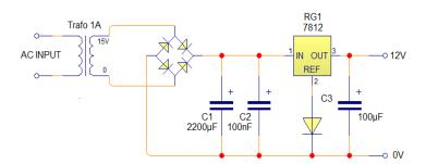
Figure 3. Low-frequency charger circuit schematic
