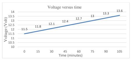
Figure 7. Graph between time and battery voltage for low-frequency charger
