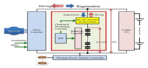
Figure 2. Battery discharging system
