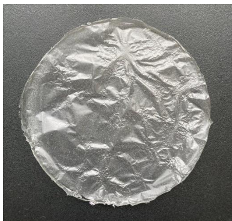
Figure 1. Physical photo of the synthesized CS-CMC/SiO 2 membrane.
